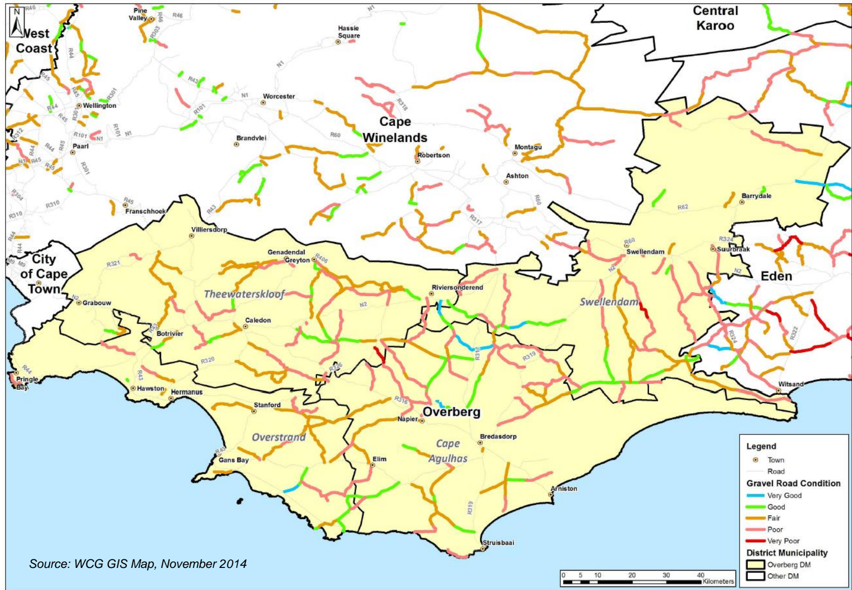
Figure 3.13: Condition of Gravel Road Network in ODM
