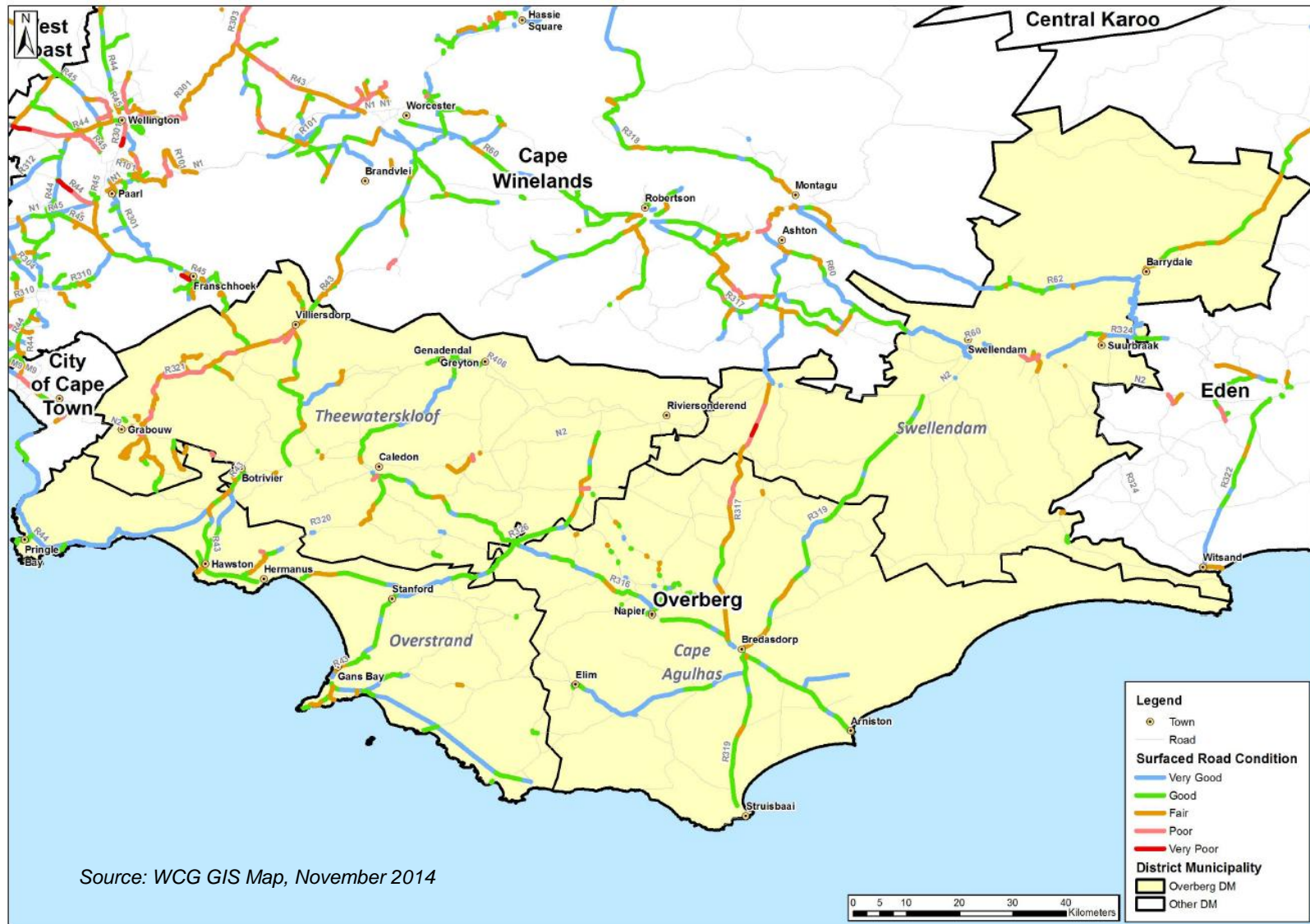
Figure 3.12: Paved road network surface condition
